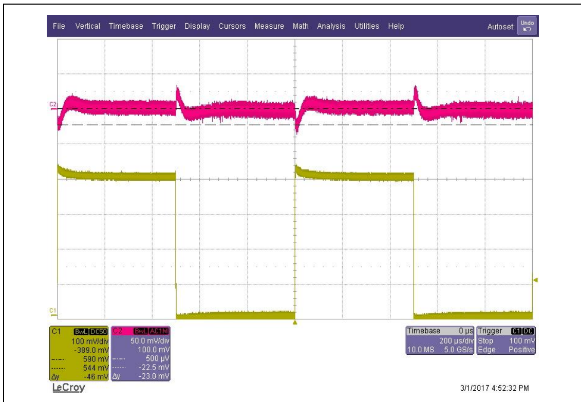
Figure 7. PVDD1=24V, load step 0mA to 400mA to 0mA, 3.3V power waveform in forced PWM mode
